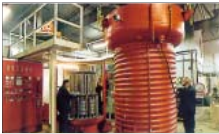
Ion nitriding plant
