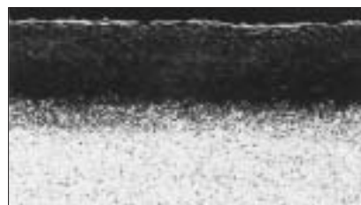
Nitrided case shown at a magnification of 100X Uddeholm Orvar 2 Microdized
