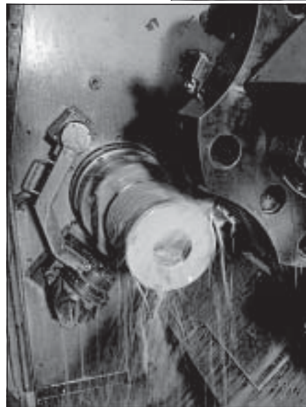
CNC-turning of dummy block in heat treated condition.
