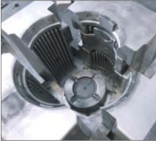
Cavity part for high pressure aluminium die casting.
