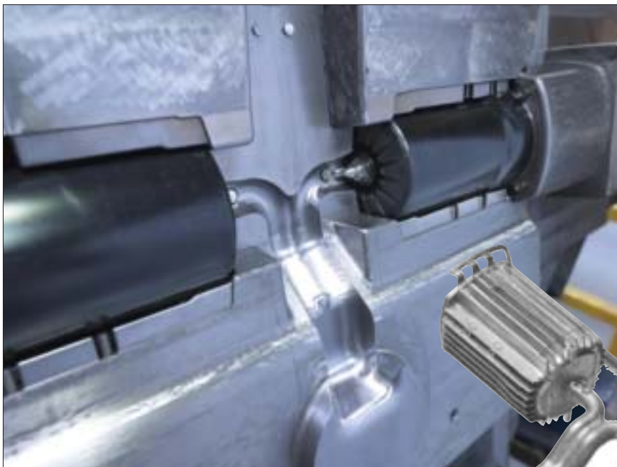
Aluminium pump housing fixed to the filling system, i.e. runners, gates and overflows.
