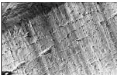
Photo 2. SEM photograph of a D2 punch worn by adhesive wear (work material austenitic stainless steel).
