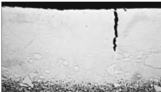
Photo 4. Surface of Uddeholm Sverker 21 after rough spark EDM. The white layer is brittle and contains cracks.
