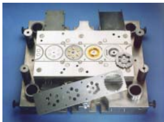
Fine blanking. Courtesy of Feintool, Switzerland
