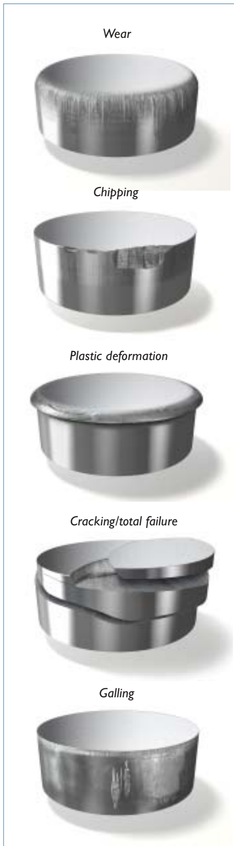
Figure 3. The most frequent failure mechanisms in cold work tooling.
