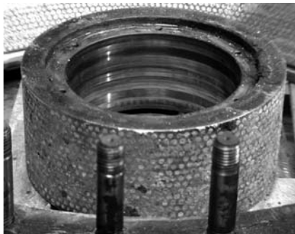
Figure 2: Matrix for manufacturing of pellets
