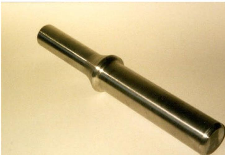
*Mandrels  $\varnothing$  203 mm are manufactured at Uddeholm Machining from hardened Orvar 2M.*
